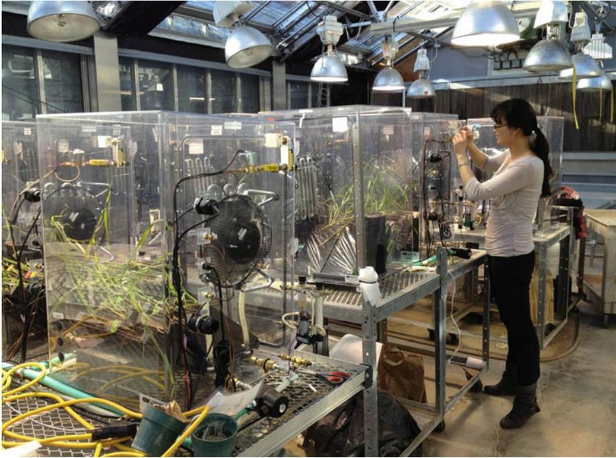
**Fig. 2.1** Plant  $e\text{CO}_2$ /isotope chambers at the EPIC facility at the University of California, Berkeley. The 16 replicate plant growth chambers pictured here are used for full-factorial experiments with controlled light, moisture, isotope, and atmospheric  $\text{CO}_2$  concentrations
